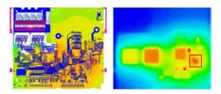
Coupling ANSYS Icepak with ANSYS SIwave (left) provides additional insight into local hotspots (right) from copper resistive losses in PCBs and packages.
