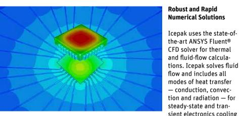
Temperature contours on micro lead-frame plastic quad (MLPQ) package in natural convection chamber sient electronics cooling applications. The solver provides complete mesh flexibility for conjugate heat transfer; it allows you to solve even the most complex electronic assemblies using unstructured meshes.
