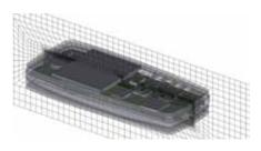
Multi-level hex-dominant mesh of cell phone assembly; hanging-node mesh resolves small geometric details.
