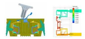
Schneider Electric used Icepak for thermal and electrical simulations on a wiring system switch device assembly to determine temperature and define conductor and insulator specifications.
